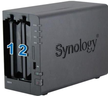
7 Replace the hard drive bay cover to finish the installation.
