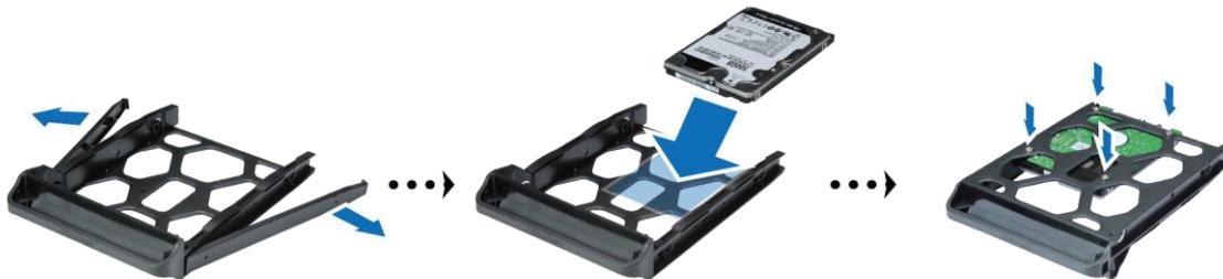
4 Make sure the side marked with "UP" is facing up, and insert the hard drive tray into the empty hard drive bay. You should hear a click when the tray is locked in place.
